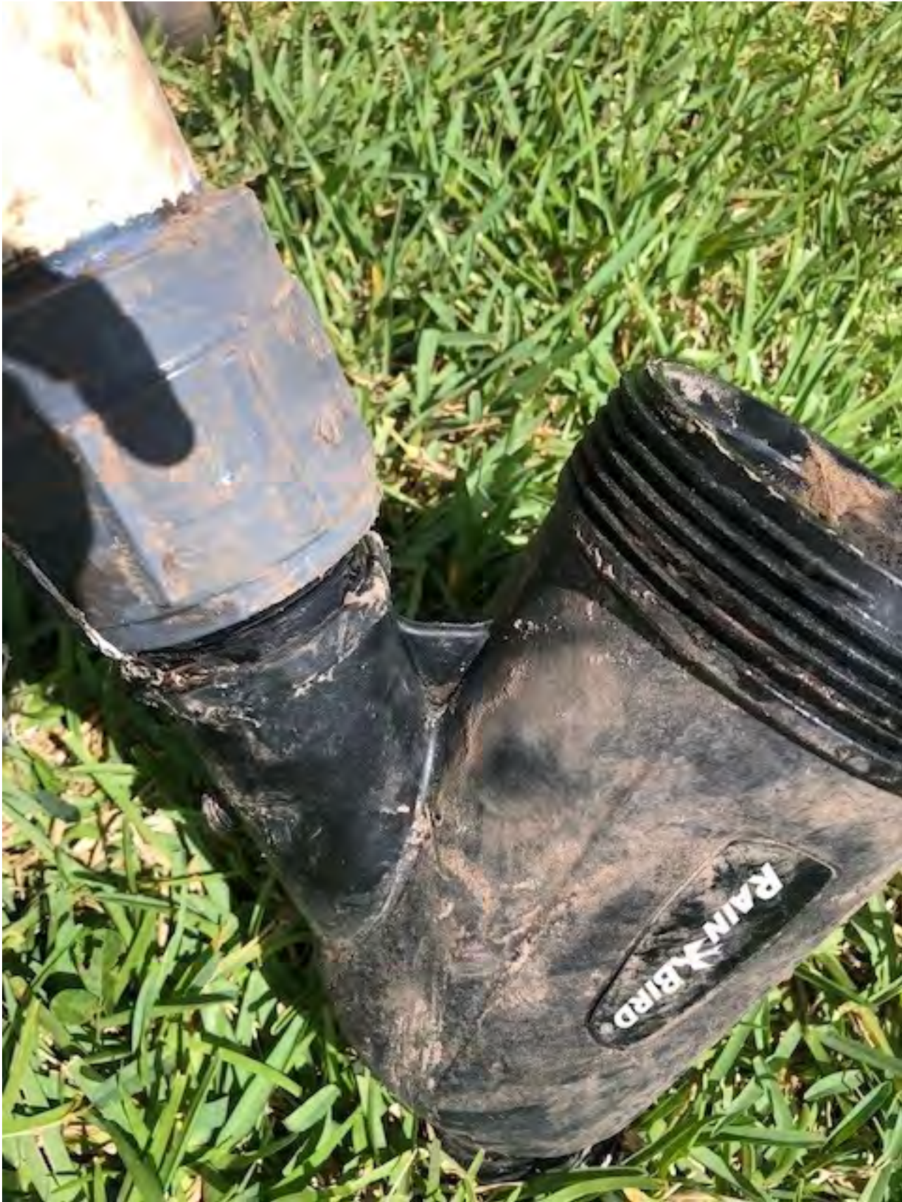
Cracked filter that led to mainline leak on Pleasant Plains.
